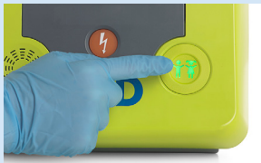
Push the Child button to invoke paediatric heart analysis algorithm and reduce energy delivered.
