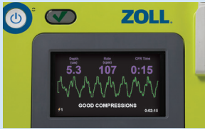
Display screen shows current rescue information and ECG in real time.
